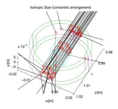
Figure 8.6: An l-4He sample in a cryostat, simulated with the Isotropic\_Sqw component in concentric geometry.
