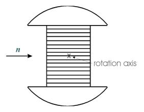
Figure 6.6: geometry of a staight Fermi chopper
