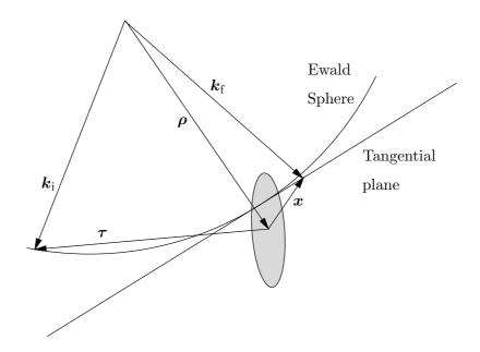
Figure 8.5: The scattering triangle in the single crystal.
