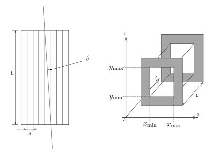
Figure 4.1: The geometry of a simple Soller blade collimators: The real Soller collimator, seen from the top (left), and a sketch of the component **Soller** (right). The symbols are defined in the text.
