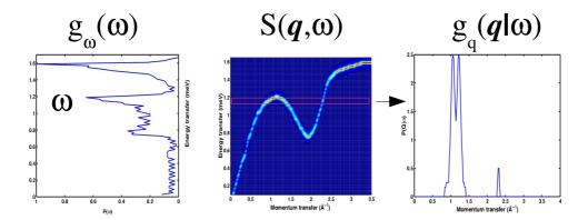
Figure 8.7: Centre: Model of dynamic structure factor  $S(q,\omega)$  for l-<sup>4</sup>He; left: probability distribution  $g_{\omega}$  (horizontal axis) of energy transfers (vertical axis, density of states); right: probability distribution  $g_q(\omega)$  (vertical axis) of momentum transfers (horizontal axis) for a given energy transfer  $\hbar\omega \sim 1.1$  meV.
