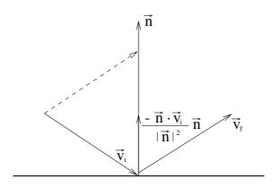
Figure 5.3: Neutron reflecting from mirror.  $\mathbf{v}_i$  and  $\mathbf{v}_f$  are the initial and final velocities, respectively, and  $\mathbf{n}$  is a vector normal to the mirror surface.
