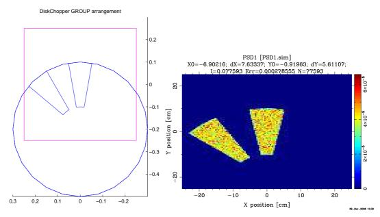
Figure 6.2: mcdisplay rendering and monitor output from a DiskChopper GROUP
